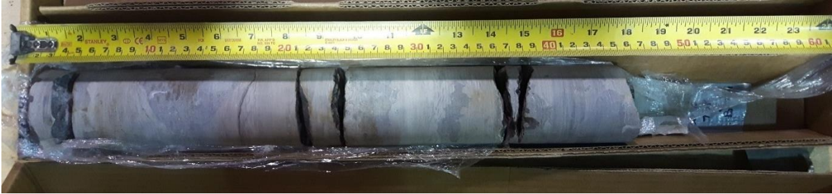
Photo 1. Core Sample for BH3 from Elevation 199.58 m to 199.17 m
