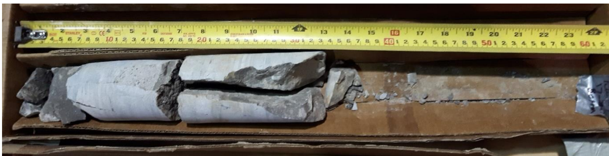
Photo 4. Core Sample for BH1 from Elevation 199.77 m to 199.36 m
