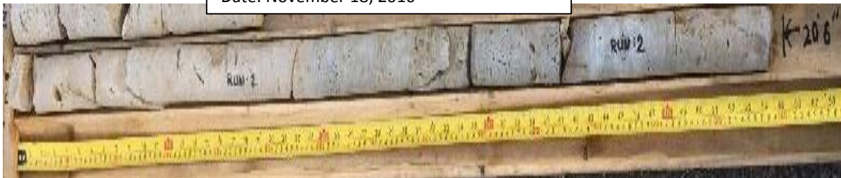
Photo 2. Core Sample(Run 2) for BH 4 from Elevation 343.1 m to 341.63 m
