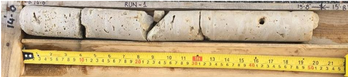
Photo 1. Core Sample(Run1) for BH 4 from Elevation 343.6 m to 343.1 m
