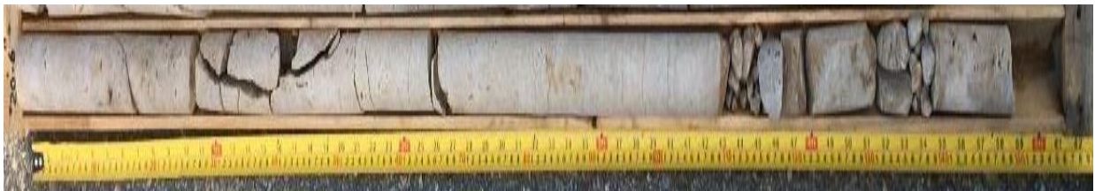
Photo 3. Core Sample(Run3) for BH 4 from Elevation 341.63 m to 340.1 m
