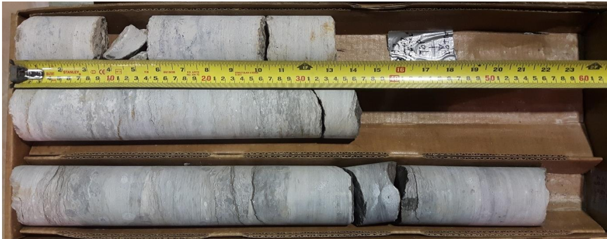
Photo 3. Core Sample for BH3 from Elevation 197.65 m to 196.43 m
