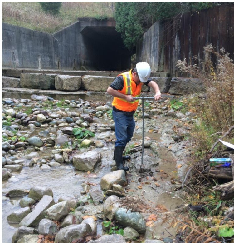
Photo 10: Probe hole using 'T' bar
