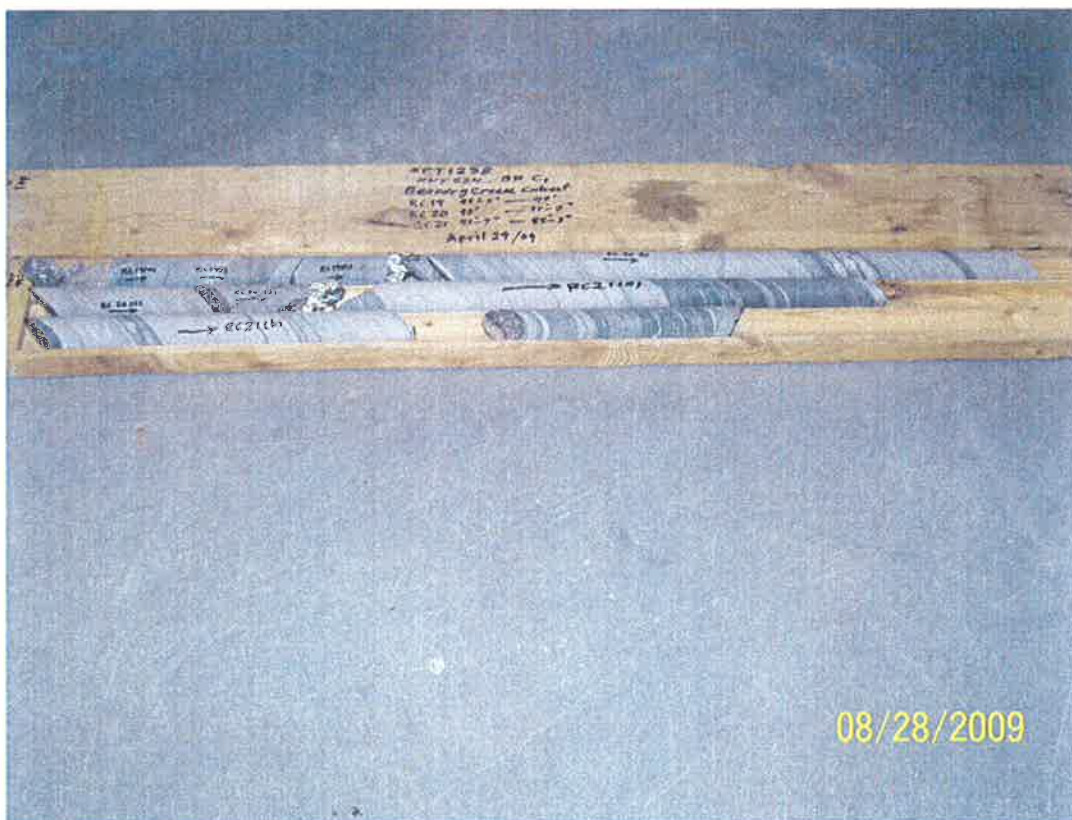
Figure D-1 -- Rock core retrieved at Borehole C1
