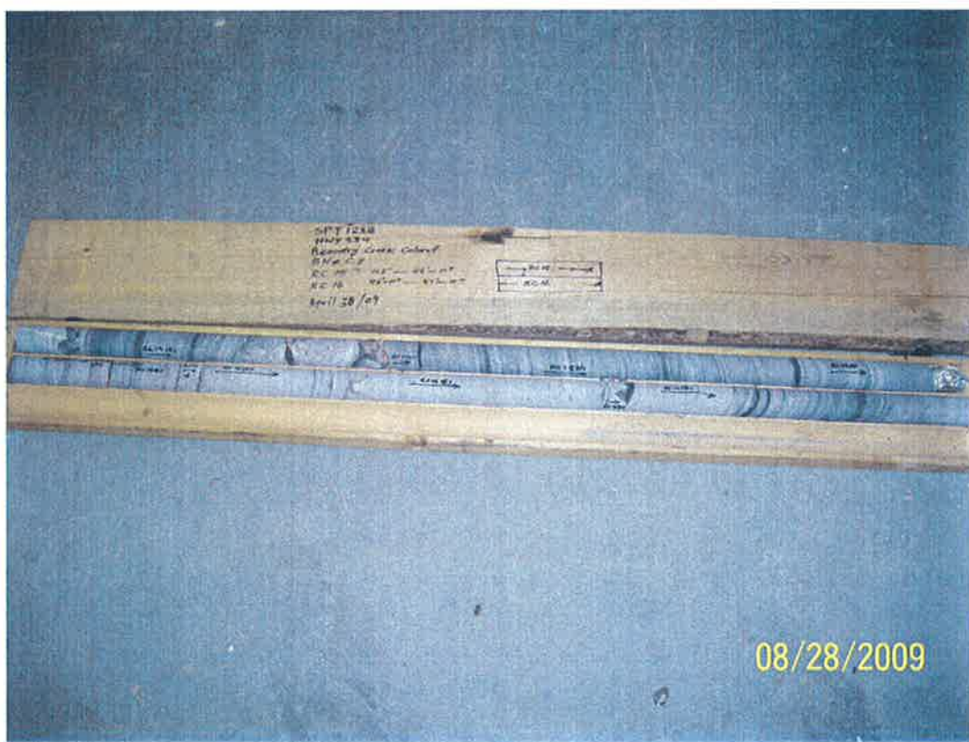
Figure D-2 -- Rock core retrieved at Borehole C2
