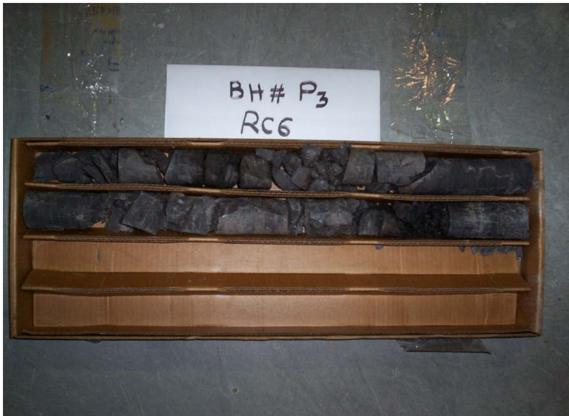
BH # P3 / Rock Core RC6, Depth (2.7 – 4.0) m
