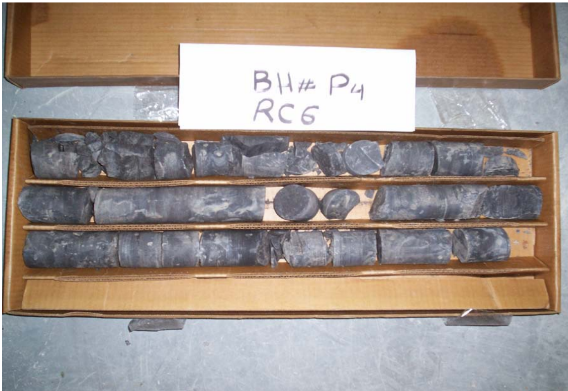
BH # P4 / Rock Core RC6, Depth (2.8 – 4.4) m
