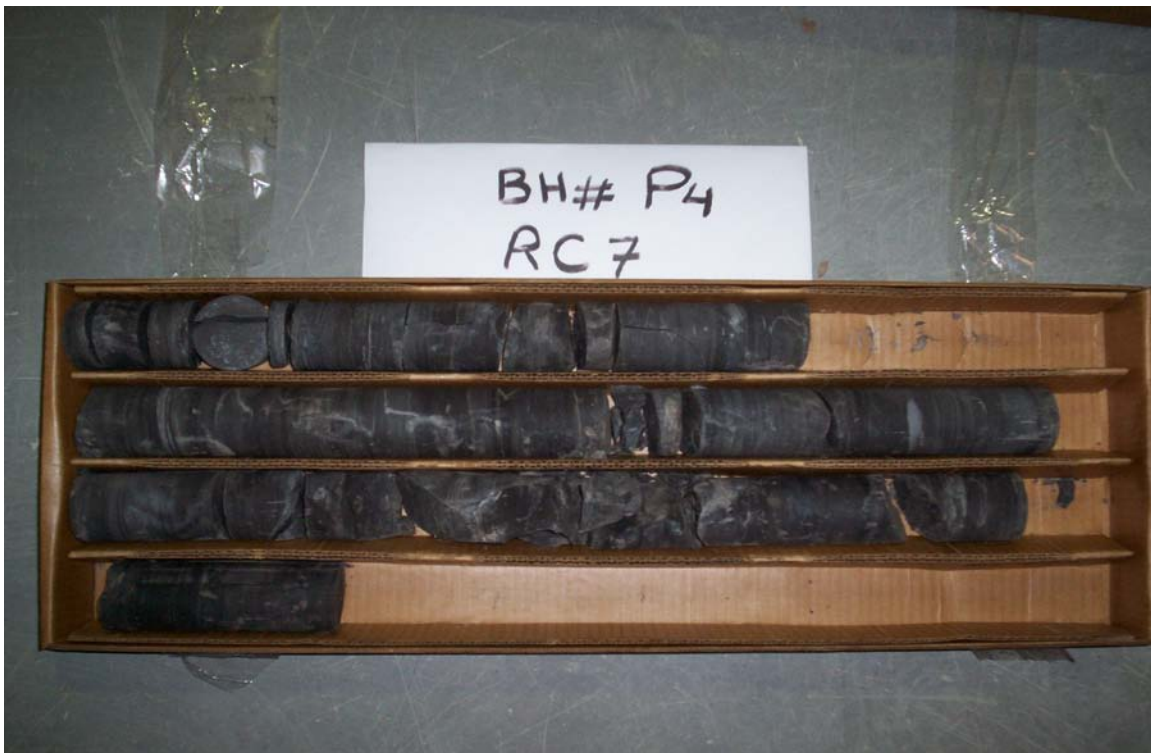
BH # P4 / Rock Core RC7, Depth (4.4 – 5.9) m
