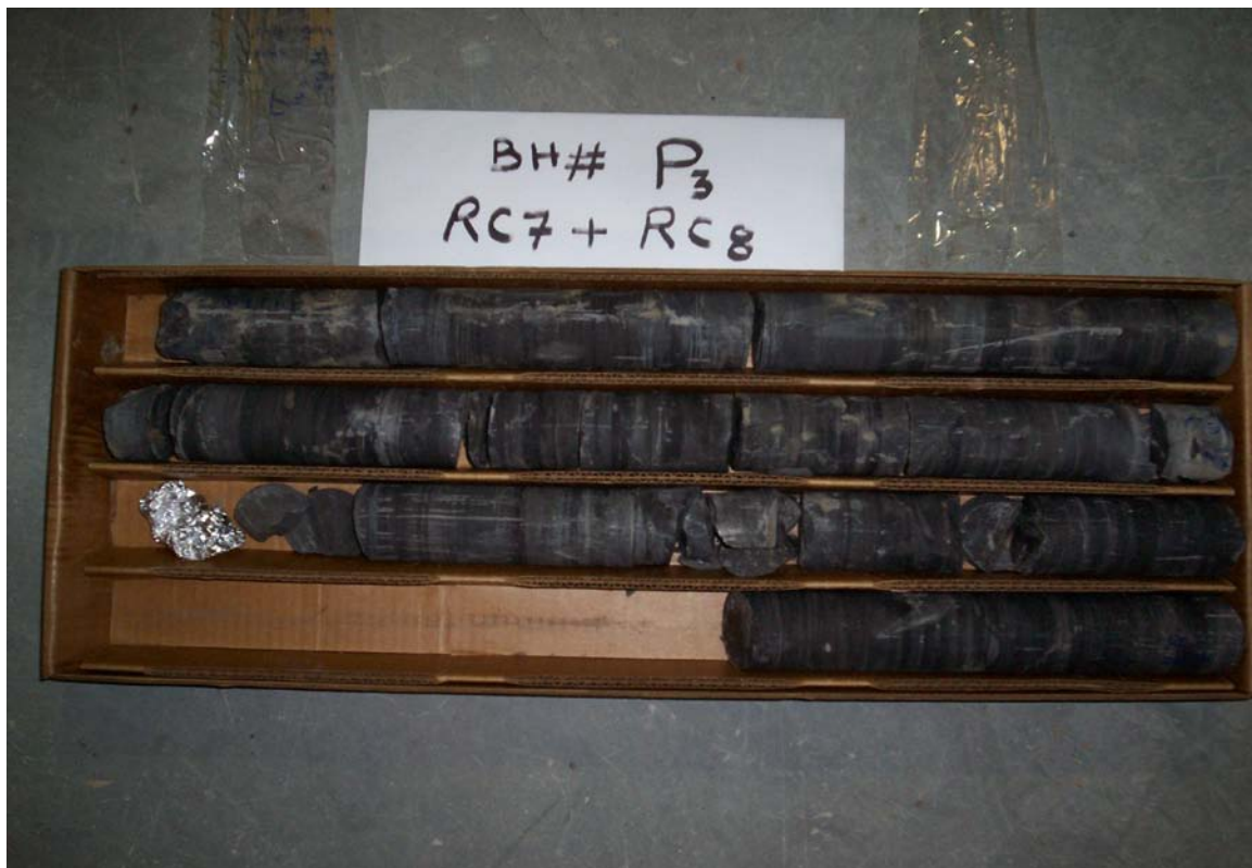
BH # P3 / Rock Core RC7 & RC8, Depth (4.0 – 5.1) m and (5.1 – 5.9) m resp.
