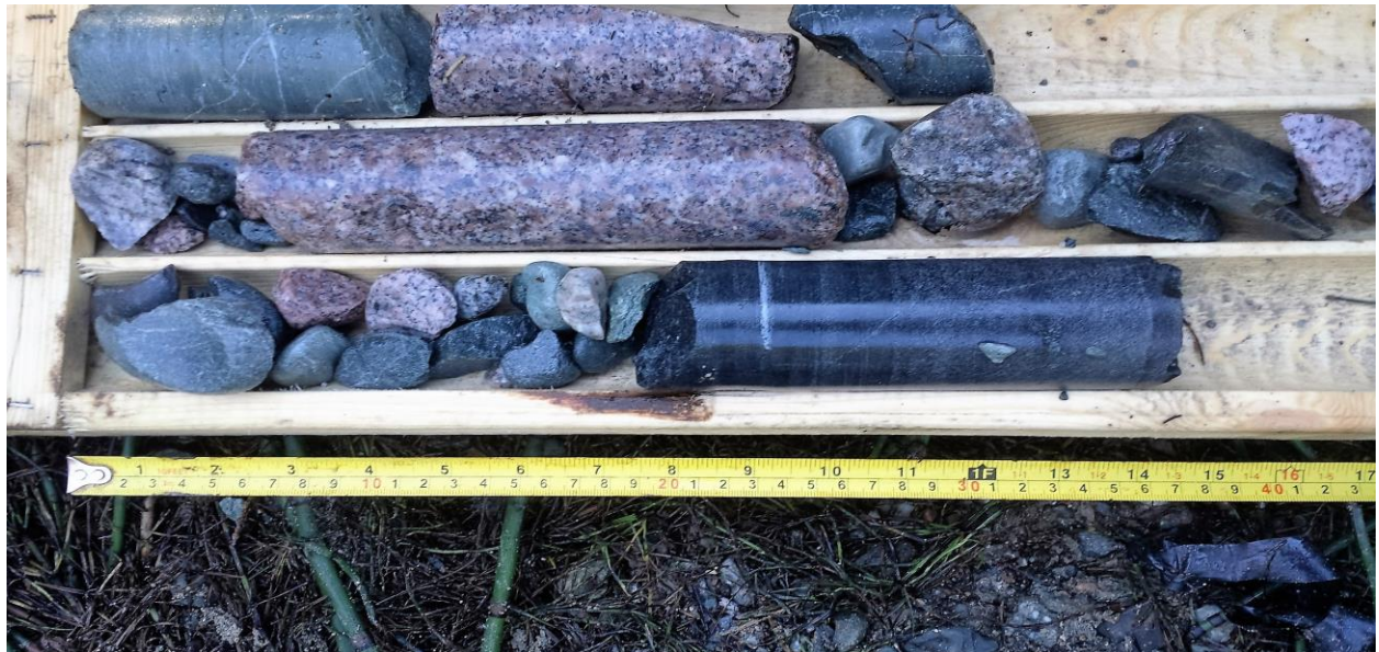
Photo 7 – Typical Sample of Cobbles and Boulders Cored in Borehole 16-01.
