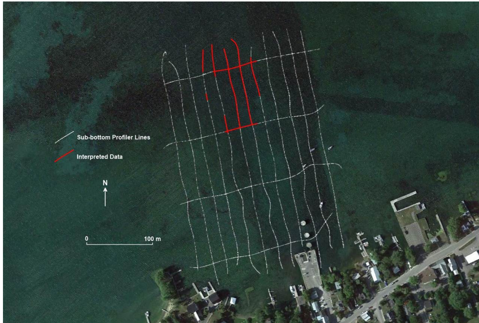
Figure 2: Site map indicating approximate sub-bottom profiler lines locations
