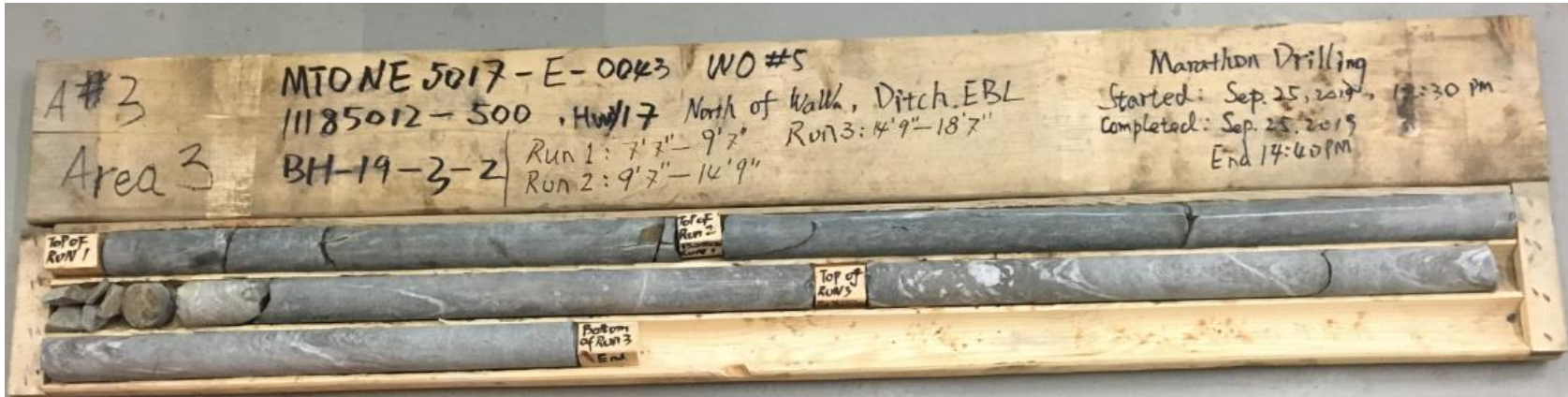
Photo 24 – Highway 17 - Area 3 - BH-19-3-02, R1 = 2.3 m – 2.8 m, R2 = 2.8 m – 4.5 m, R3 = 4.5 m – 5.7 m
