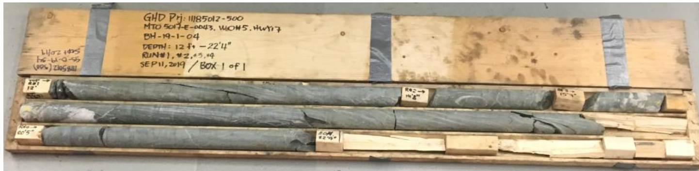
Photo 20 – Highway 17 – Area 1 - BH-19-1-04, R1 = 3.7 m – 4.4 m, R2 = 4.4 m – 4.7 m, R3 = 4.7 m – 6.2 m, and R4 = 6.2 m – 6.8 m
