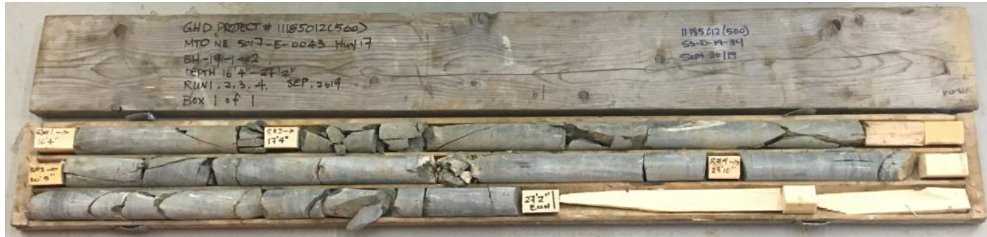
Photo 19 – Highway 17 - Area 1 - BH-19-1-02, R1 = 5.0 m – 5.4 m, R2 = 5.4 m – 6.2 m, R3 = 6.2 m – 7.3 m, and R4 = 7.3 m – 8.3 m
