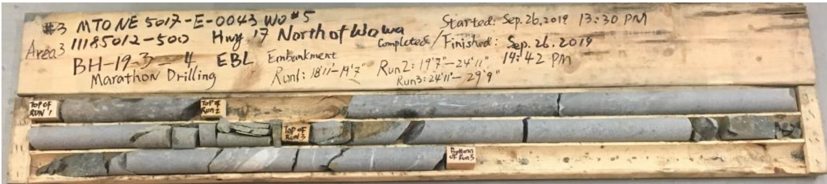
Photo 25 – Highway 17 – Area 3 - BH-19-3-04, R1 = 5.8 m – 6.1 m, R2 = 6.1 m – 7.6 m, R3 = 7.6 m – 9.1 m
