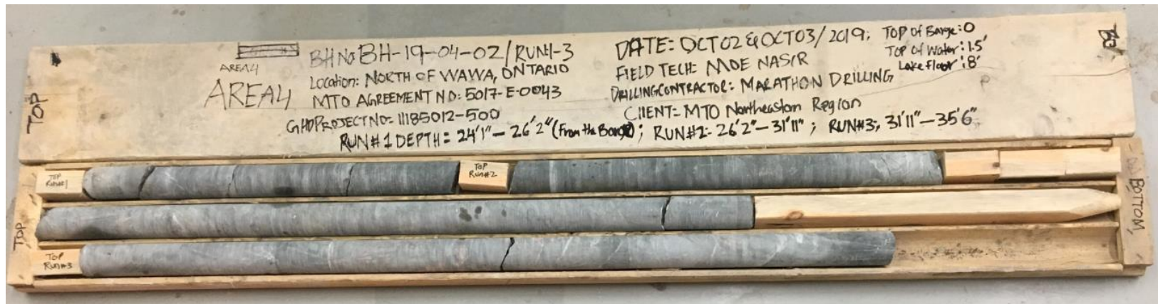
Photo 25 – Highway 17 – Area 4 - BH-19-4-02, R1 = 7.2 m – 7.8 m, R2 = 7.8 m – 9.8 m, R3 = 9.8 m – 10.8 m
