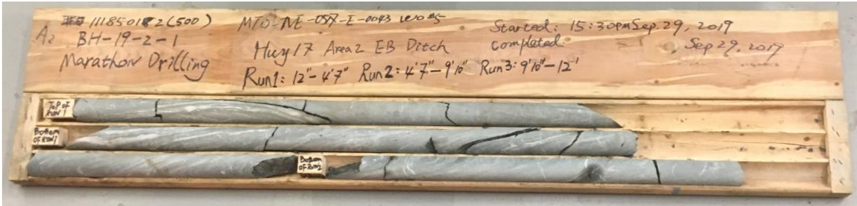
Photo 22 – Highway 17 - Area 2 - BH-19-2-01, R1 = 0.3 m – 1.4 m, R2 = 1.4 m – 3.0 m, R3 = 3.0 m – 3.7 m
