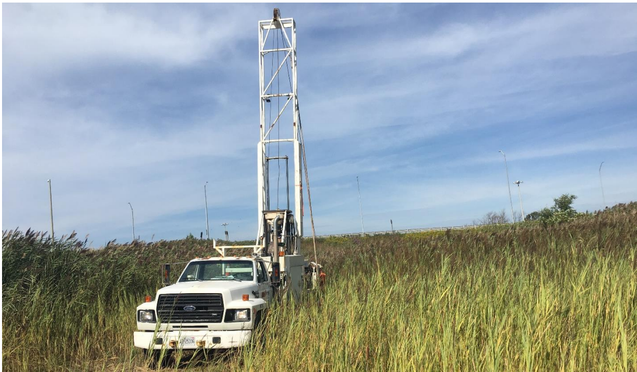
Photo C2-2 Field investigation on BH OHS8-2 with CME 55 Truck Mount Rig (Sept 2019)
