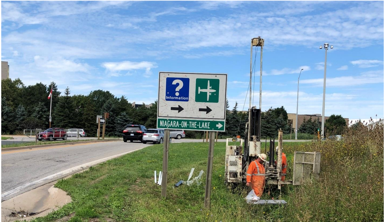
Photo C2-1 Field investigation on BH OHS1-1 with M5T Track Mount Rig (Aug 2019)
