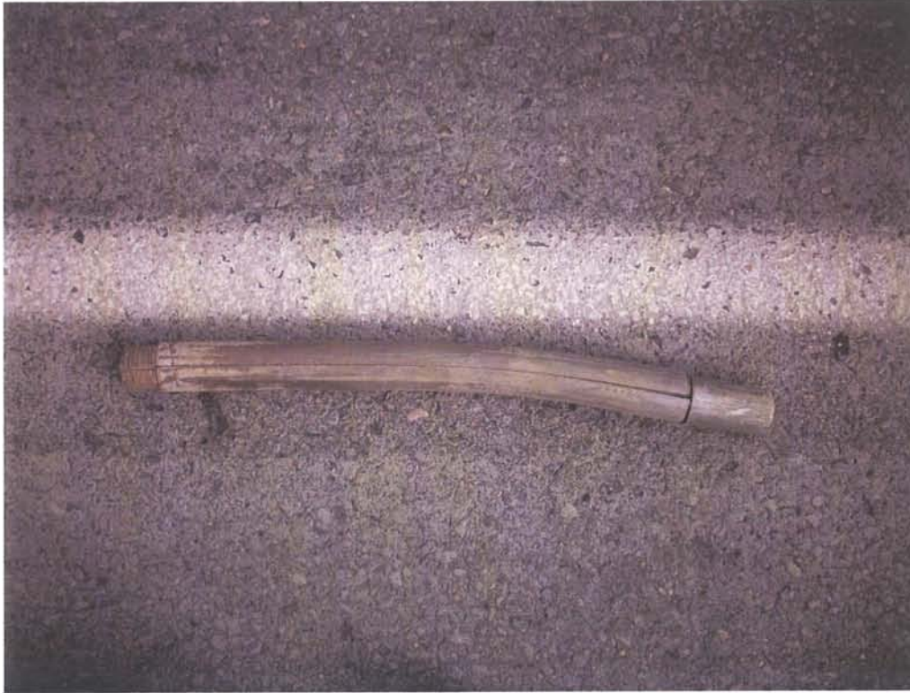
Photo No. E3: Site No. 46-395/c. Split spoon sampler that was bent trying to penetrate fill in BH 10-11 that contains cobbles and boulders.
