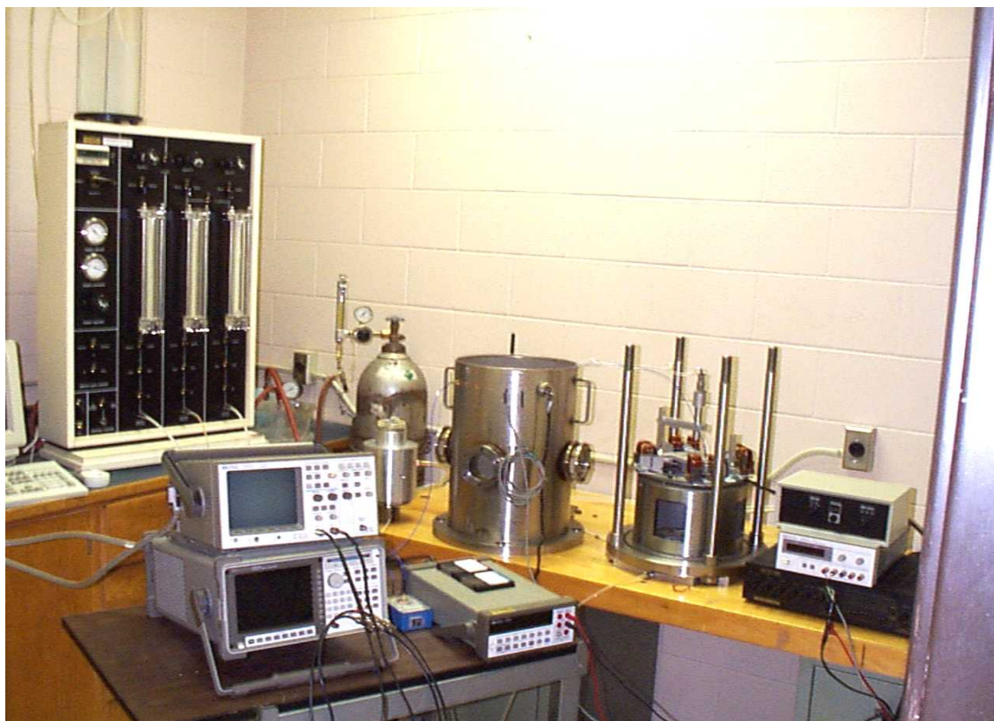
Figure 1-B. Resonant column experimental setup
