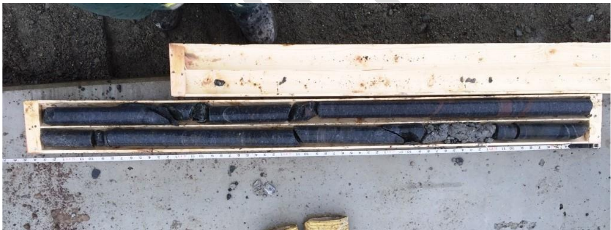
Photograph B2 – Rock core sample from Borehole 16-02
