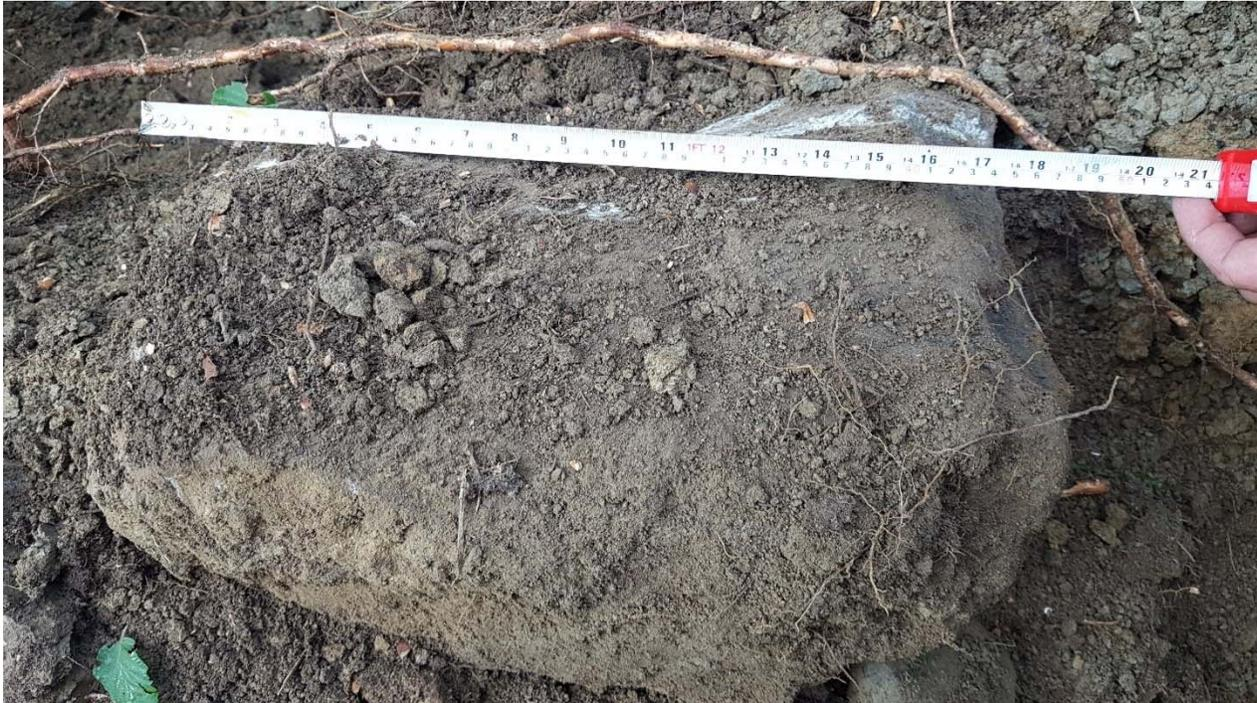
*Photograph 2: Boulder encountered while excavating TP 18-109A*
