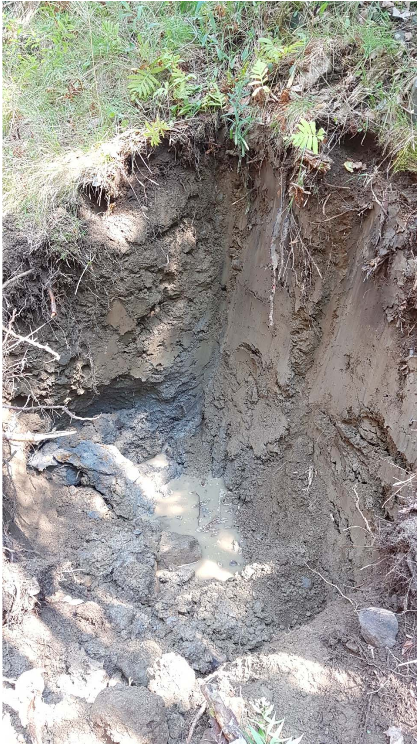
Photograph 3: Quick water ingress at TP 18-108B (looking east towards HWY 60 embankment)
