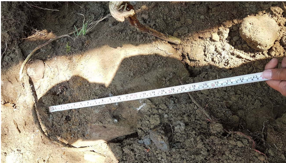
Photograph 2: Boulder encountered in the excavated soil from TP 18-108A
