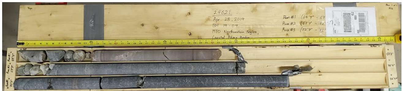
Photo B5: Borehole 19-09 core photo. Run #1 to 3.
