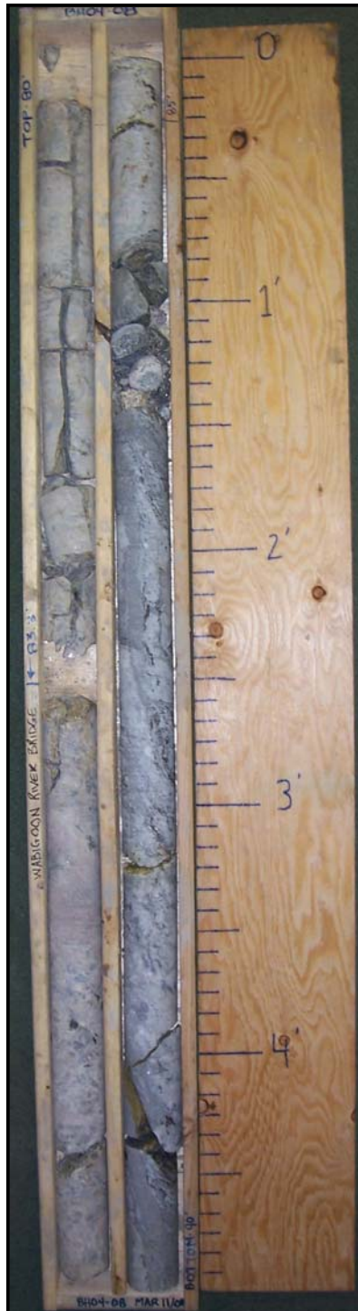
BH 4-2008 - Rock Core (from 35.0 to 37.5 m depth) Overall view and close-up views.
