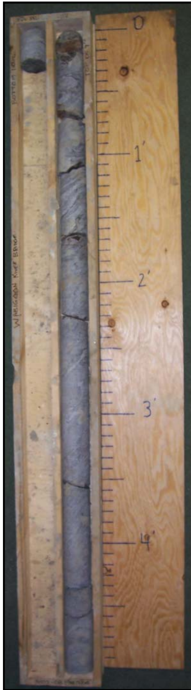
BH 2-2008 - Rock Core (from 35.0 to 37.5 m depth) Overall view and close-up views.
