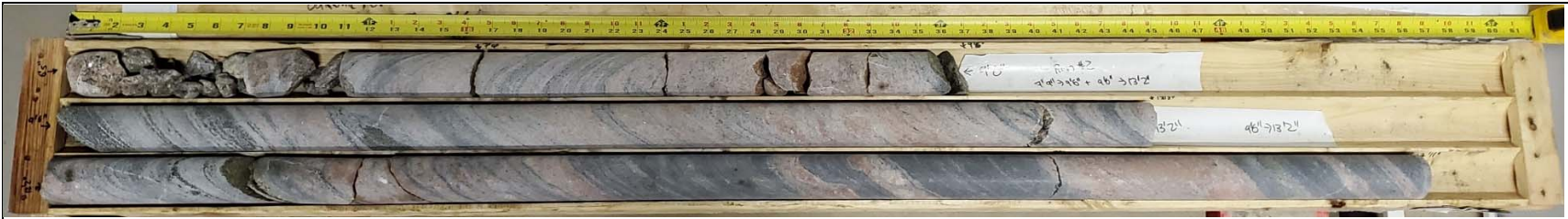
BOREHOLE: BH-01 RUN NO. 1: 2.0 m to 2.4 m RUN NO. 2: 2.4 m to 4.0 m RUN NO. 3: 4.0 m to 5.5 m
