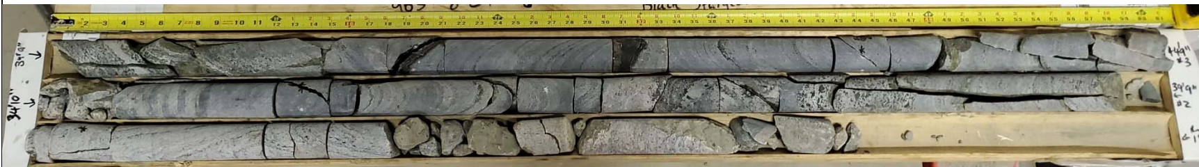
BOREHOLE: BH-02 RUN NO. 1: 8.5 m to 10.3 m (Boulders and Cobbles) RUN NO. 2: 10.6 m to 12.1 m RUN NO. 3: 12.1 m to 13.6 m
