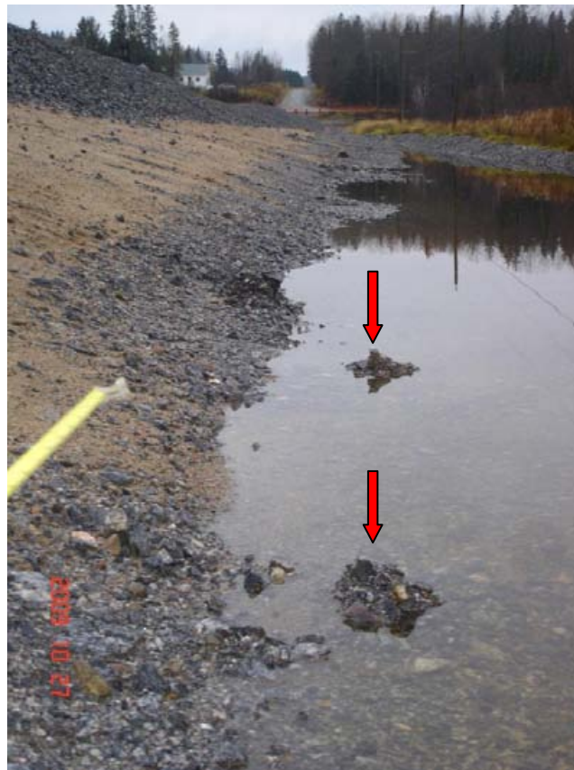
Figure E12 – More sand boils at the top of backfill in the north ditch
