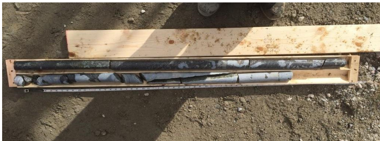
Photograph B1 – Rock core sample from Borehole 16-01
