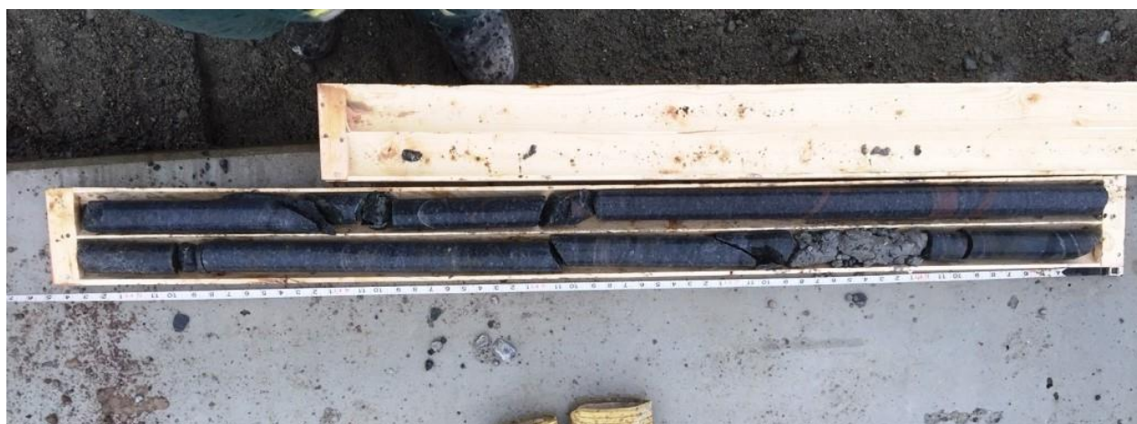
Photograph B2 – Rock core sample from Borehole 16-02
