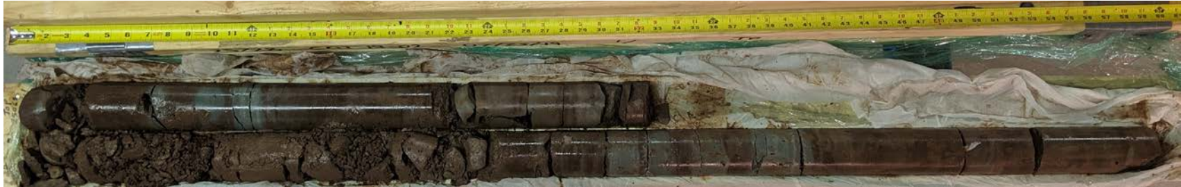
Borehole 19-44 – Run 3 – 21.34-23.01 m
