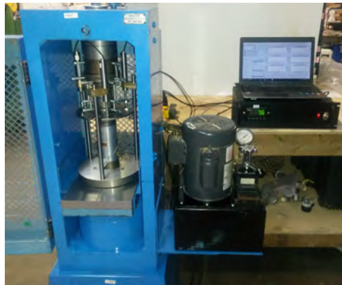
Figure 1: Forney loading frame setup for UCS testing.
