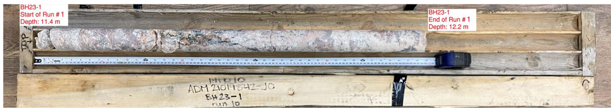
Photograph D1. Rock cores from BH23-1, Run 1 – 11. 4 m to 12.2 m (October 2023)
