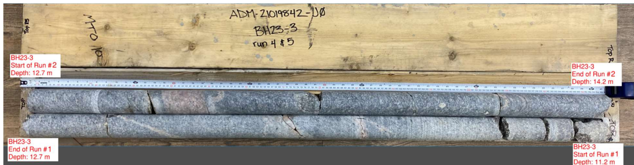
Photograph D2. Rock cores from BH23-3, Run 1 and Run 2 – 11. 2 m to 14.2 m (October 2023)
