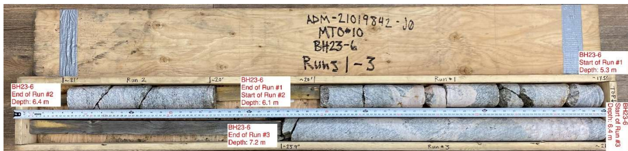
Photograph D5. Rock cores from BH23-6, Run 1 to Run 3 – 5.3 m to 7.2 m (October 2023)
