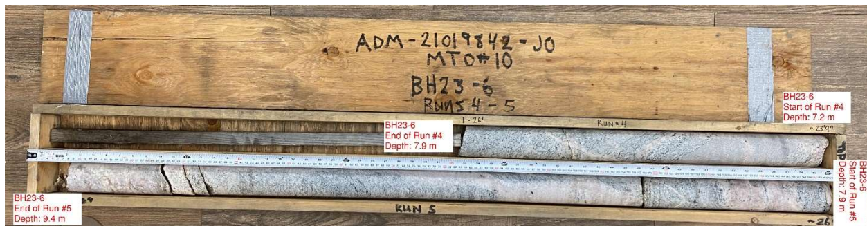
Photograph D6. Rock cores from BH23-6, Run 4 and Run 5 – 7.2 m to 9.4 m (October 2023)
