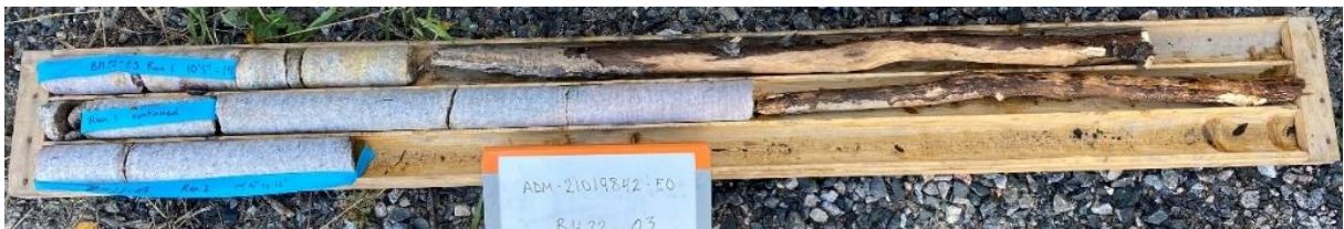
Photograph E3. Bedrock core samples, BH22-03, Run 1 (top and middle) and Run 2 (bottom), October 2022
