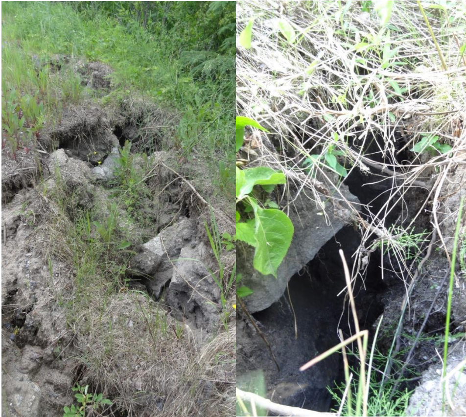
Photo 4 and Photo 5: July 7, 2022 – Tension Cracks Directly West of Highway 658 within Slope Instability
