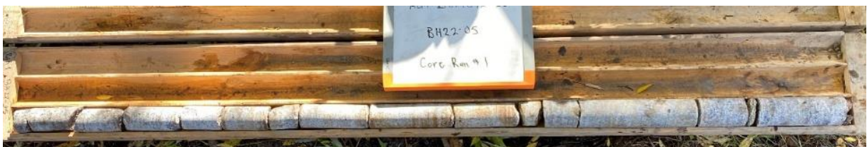
Photograph E4. Bedrock core samples, BH22-05, Run 1, October 2022
