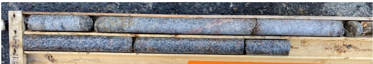
Photograph E2. Bedrock core samples, BH22-02, Run 1 (top) and Run 2 (bottom), October 2022
