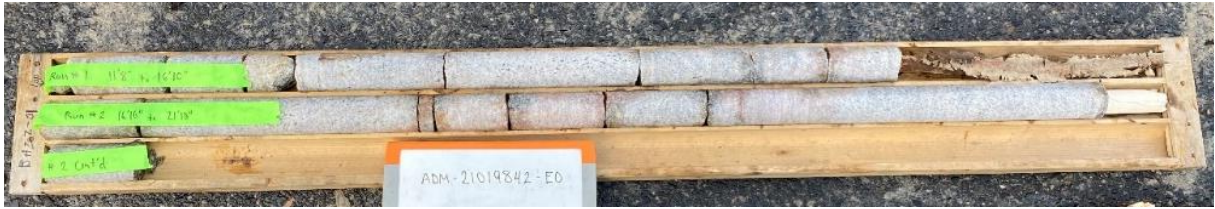
Photograph E1. Bedrock core samples, BH22-01, Run 1 (top) and Run 2 (middle and bottom), October 2022
