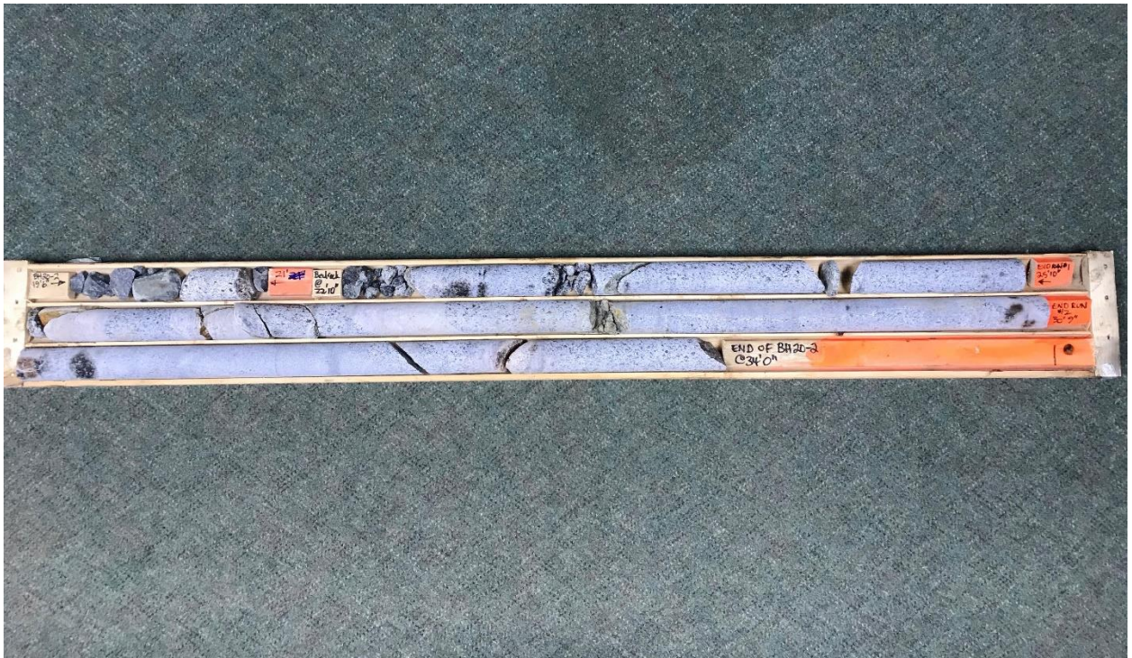
Photograph E2. Bedrock core samples, borehole BH20-2, November 2020
