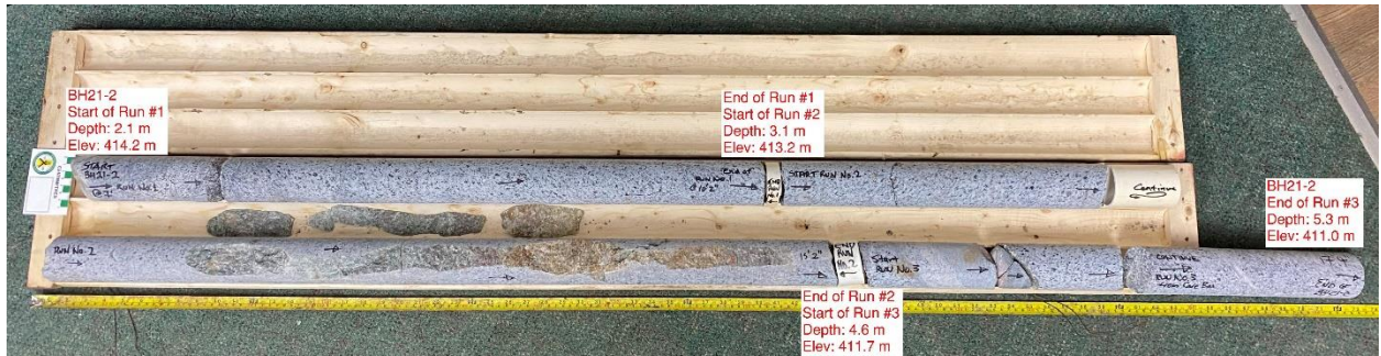
Photograph E3. Bedrock Core Samples, Borehole BH21-2 , November 2021
