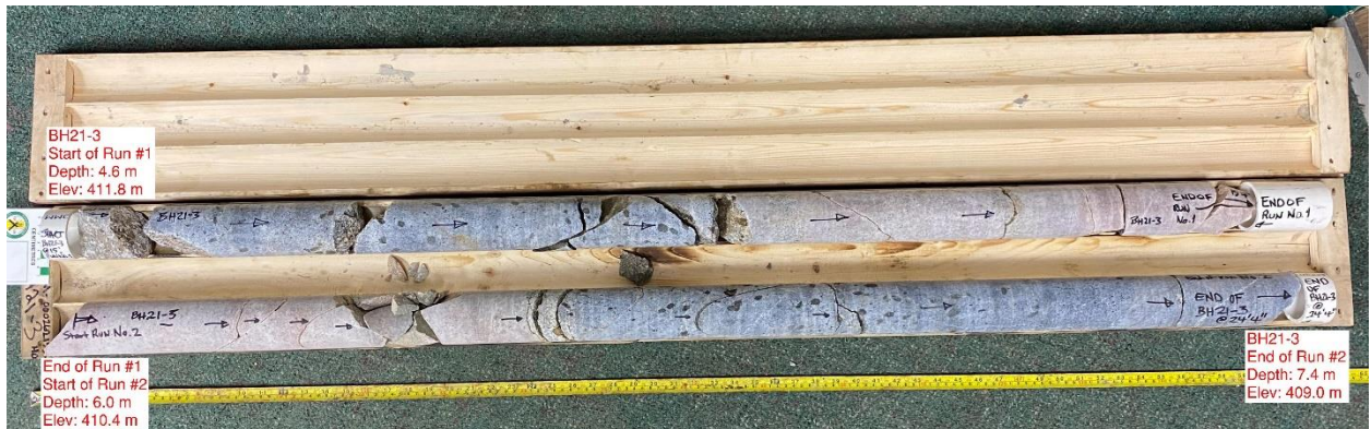
Photograph E4. Bedrock Core Samples, Borehole BH21-3 , November 2021
