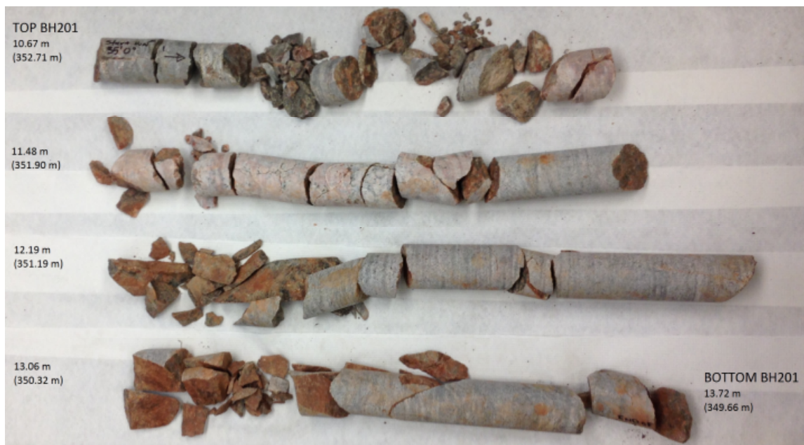
BH201 - Bedrock Core Samples with Depths and Elevations
