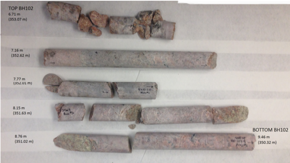
BH102 - Bedrock Core Samples with Depths and Elevations
