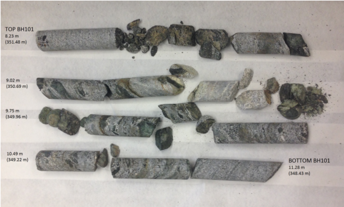
BH101 - Bedrock Core Samples with Depths and Elevations
