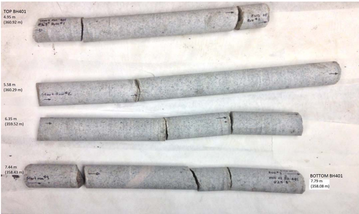
BH401 - Bedrock Core Samples with Depths and Elevations
