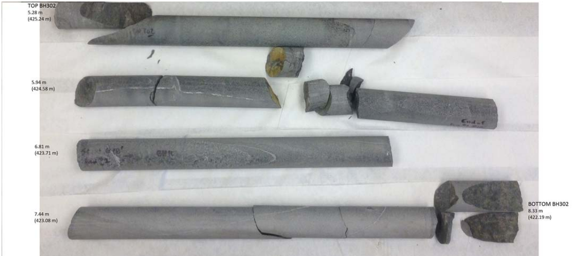
BH302 - Bedrock Core Samples with Depths and Elevations
