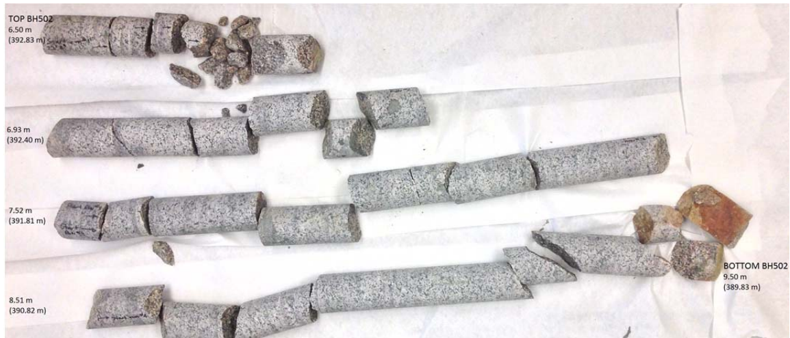
BH502 - Bedrock Core Samples with Depths and Elevations
