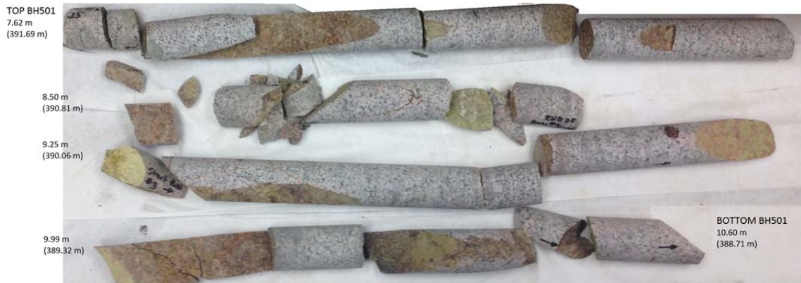
BH501 - Bedrock Core Samples with Depths and Elevations
