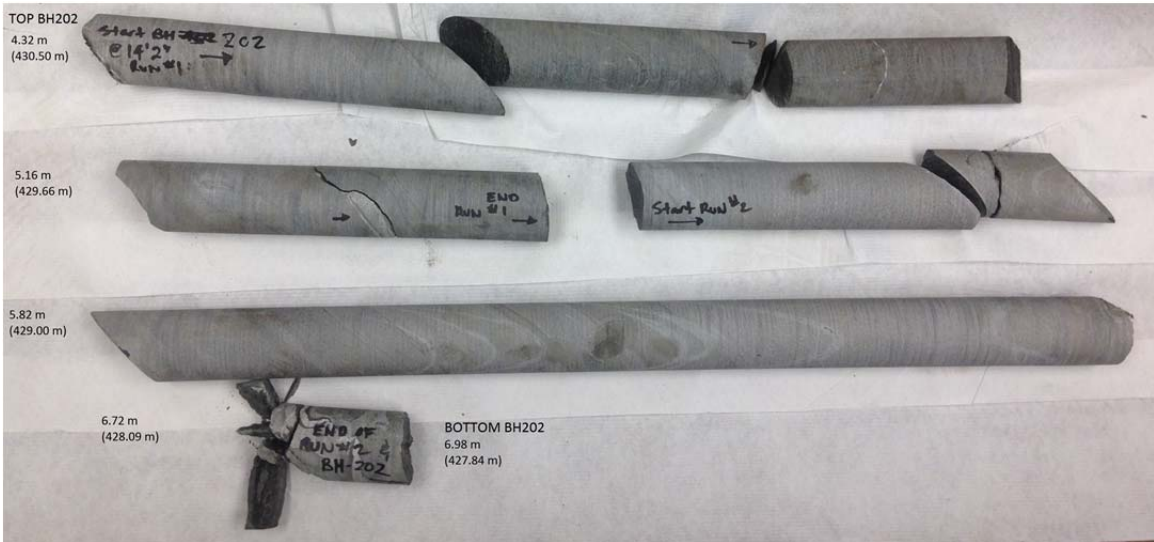
BH202 - Bedrock Core Samples with Depths and Elevations
