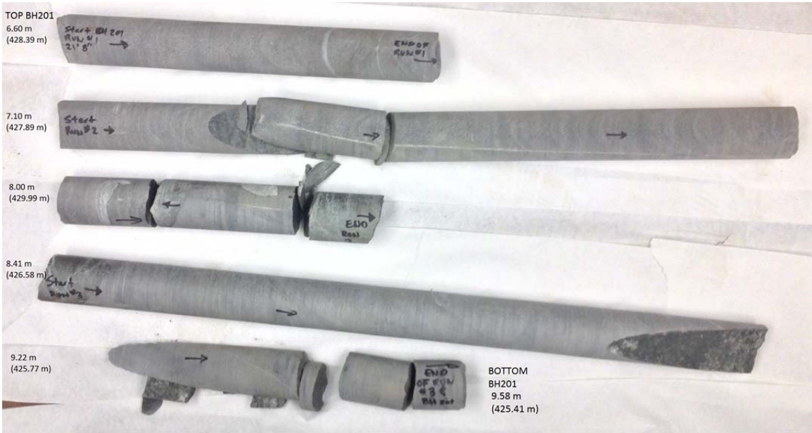
BH201 - Bedrock Core Samples with Depths and Elevations
