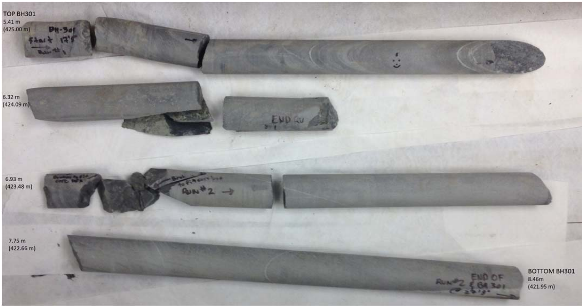
BH301 - Bedrock Core Samples with Depths and Elevations
