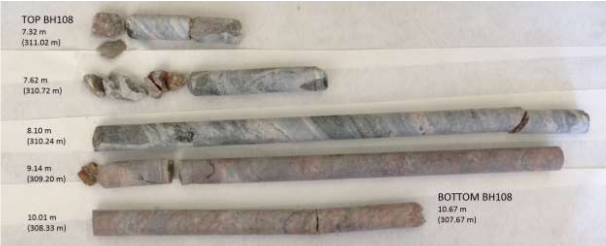
BH108 - Bedrock Core Samples with Depths and Elevations
