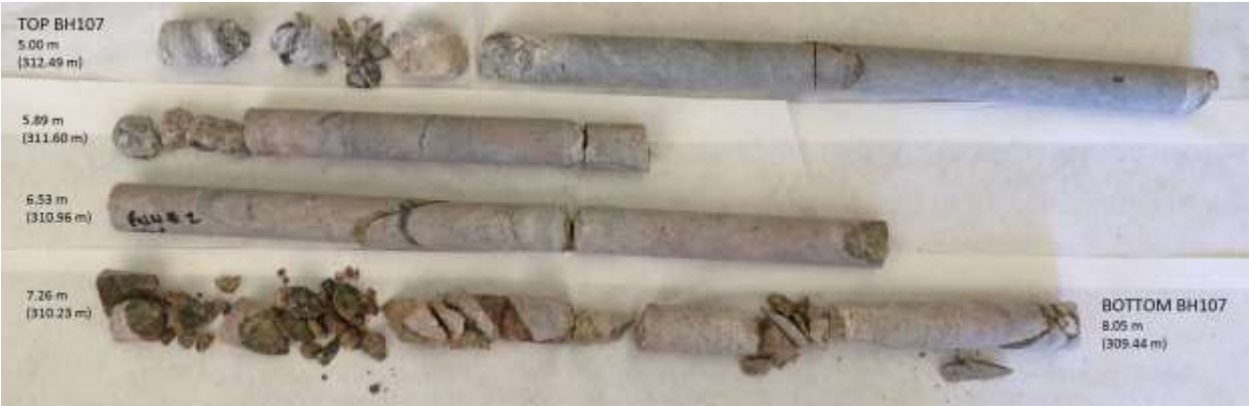
BH107 - Bedrock Core Samples with Depths and Elevations
