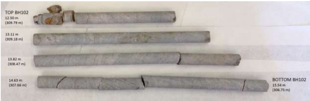
BH102 - Bedrock Core Samples with Depths and Elevations
