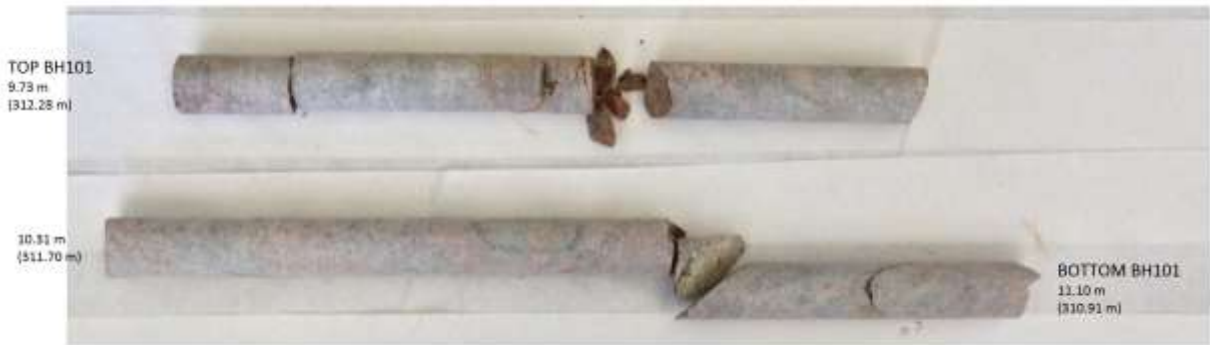
BH101 - Bedrock Core Samples with Depths and Elevations
