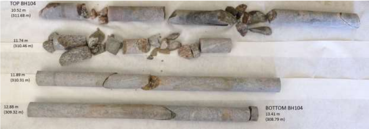
BH104 - Bedrock Core Samples with Depths and Elevations
