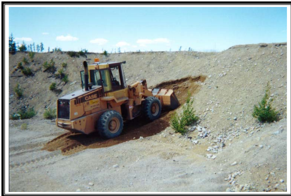
Photo 6: Sampling of the gravel source from large esker deposit.
