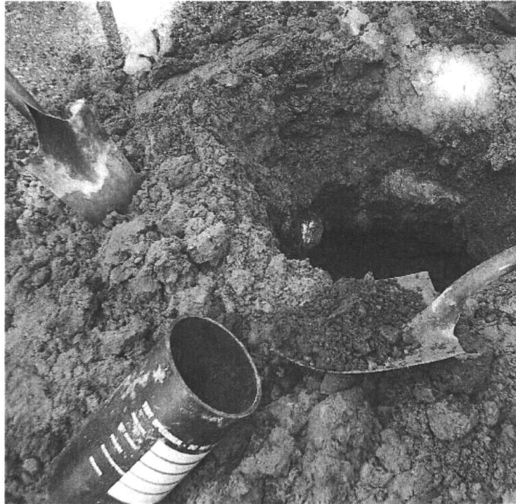
Typical Granular Sub-base Sample taken from side of Test Hole
