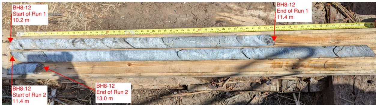
Photograph E8. Rock cores from BH8-12. Top: Run 1, Middle/Bottom: Run 2.
