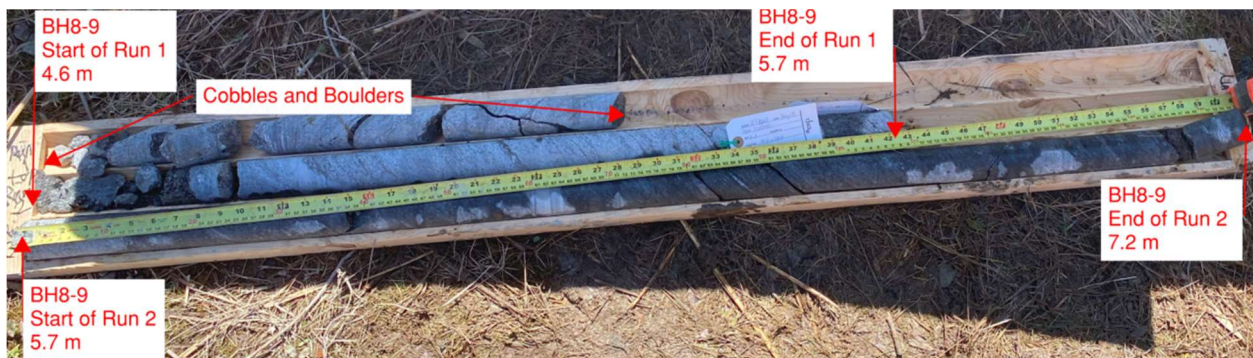
Photograph E6. Rock cores from BH8-9. Top: Cobbles and Boulders, Middle: Run 1, Bottom: Run 2.
