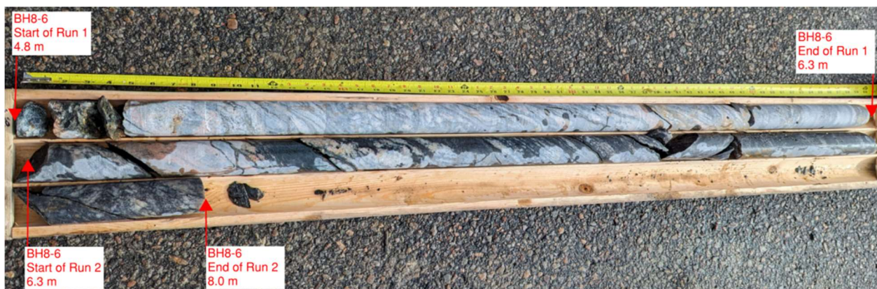
Photograph E3. Rock cores from BH8-6. Top: Run 1, Middle/Bottom: Run 2.
