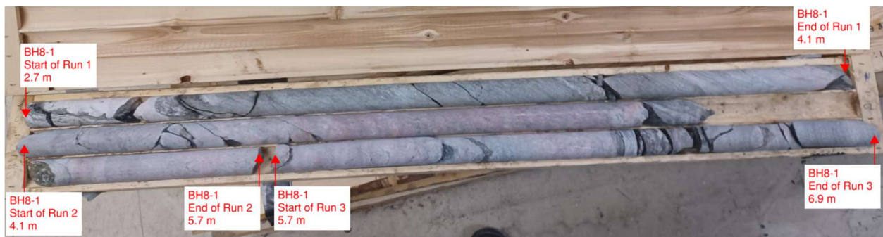
Photograph E1. Rock cores from BH8-1. Top: Run 1, Middle/Bottom: Run 2, Bottom: Run 3.
