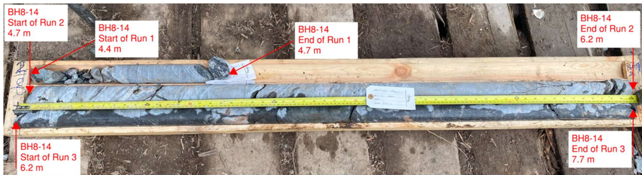
Photograph E10. Rock cores from BH8-14. Top: Run 1, Middle/Bottom: Run 2.
