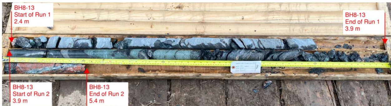
Photograph E9. Rock cores from BH8-13. Top: Run 1, Middle/Bottom: Run 2.
