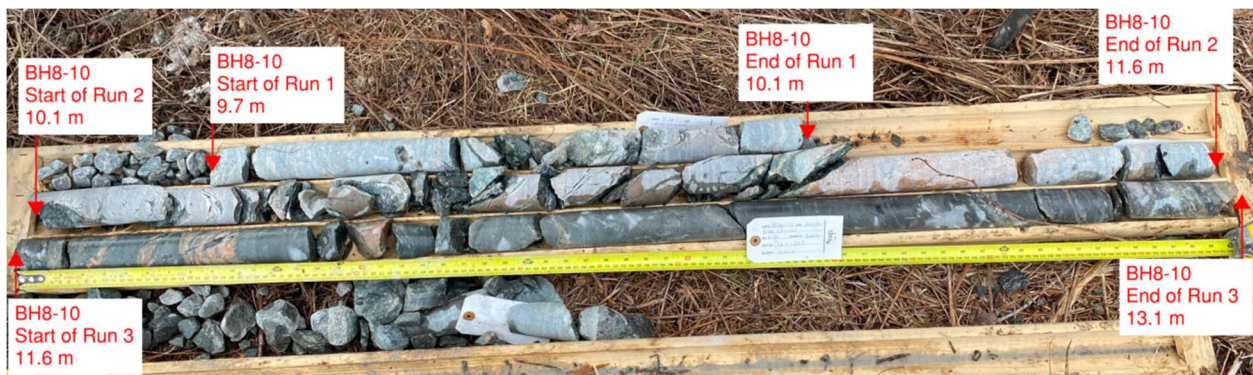
Photograph E7. Rock cores from BH8-10. Top: Run 1, Middle: Run 2, Bottom: Run 3.
