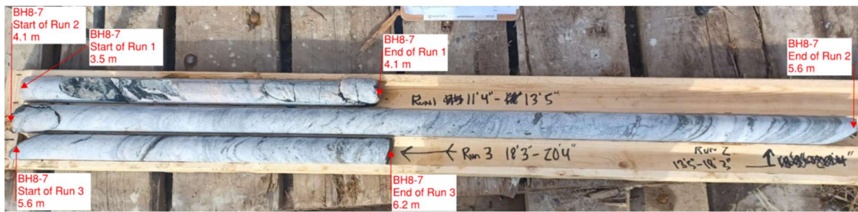
Photograph E4. Rock cores from BH8-7. Top: Run 1, Middle: Run 2, Bottom: Run 3.
