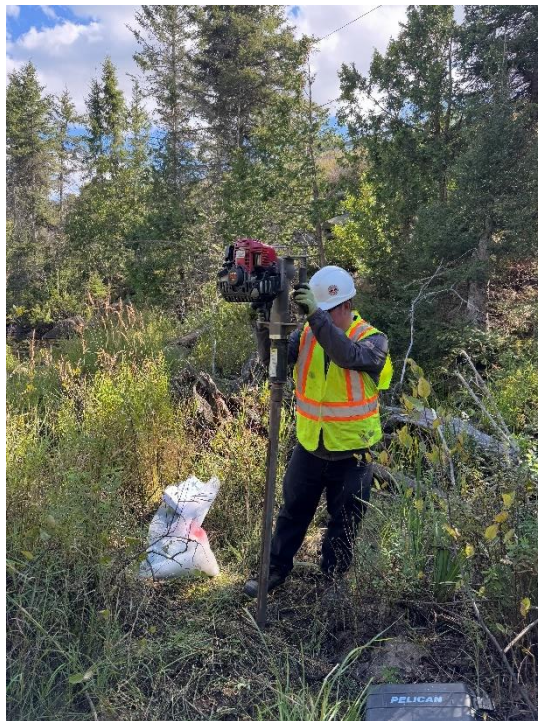
Photograph 6. Honda GX35 Portable Soil Sampler used for the probeholes on the east side of the embankment
