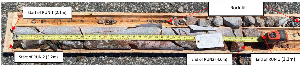
Photograph E3. Rock cores from BH12-4. Middle: Run 1, Bottom: Run 2.
