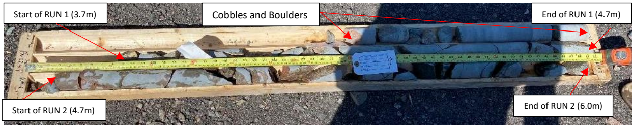
Photograph E7. Rock cores from BH12-15. Middle: Run 1, Bottom: Run 2.
