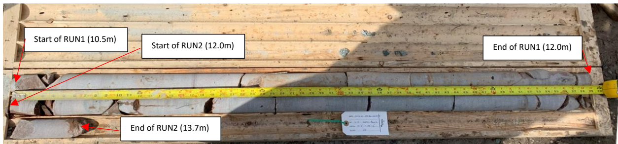
Photograph E2. Rock cores from BH12-3. Top: Run 1, Middle/Bottom: Run 2.
