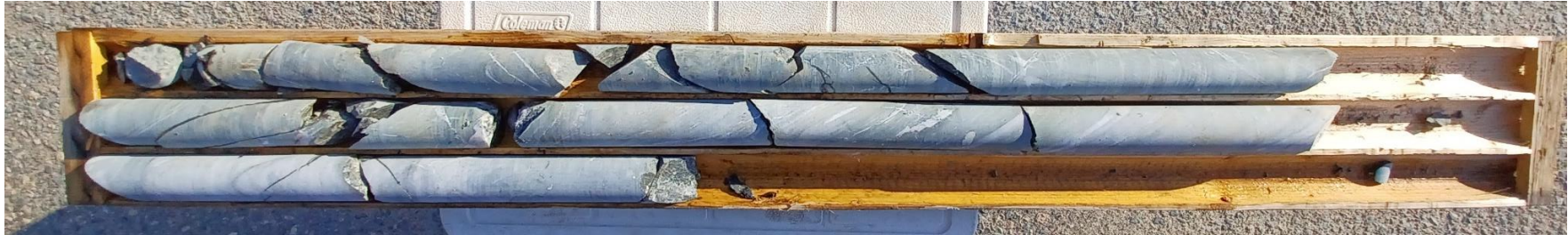
Figure E1. Bedrock core samples, 23-ST-1, Run 1 (top), Run 2 (middle), Run 3 (bottom), October 3, 2023
