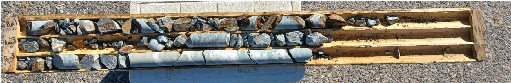
Figure E2. Bedrock core samples, 23-ST-2, Run 1 (top), Run 2 (middle), Run 3 (bottom), October 3, 2023
