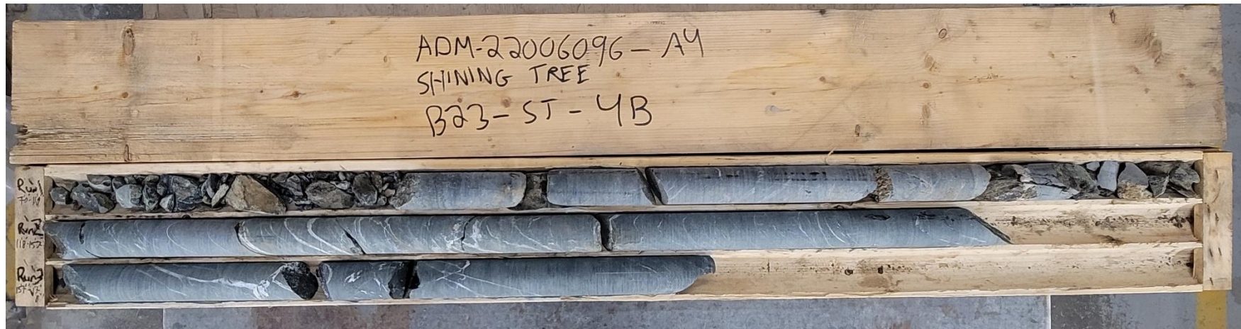
Figure E4. Bedrock core samples, 23-ST-4B, Run 1 (top), Run 2 (middle), Run 3 (bottom), October 6, 2023
