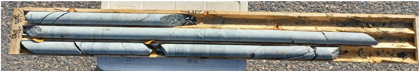
Figure E3. Bedrock core samples, 23-ST-3, Run 1 (top), Run 2 (middle), Run 3 (bottom), October 2, 2023
