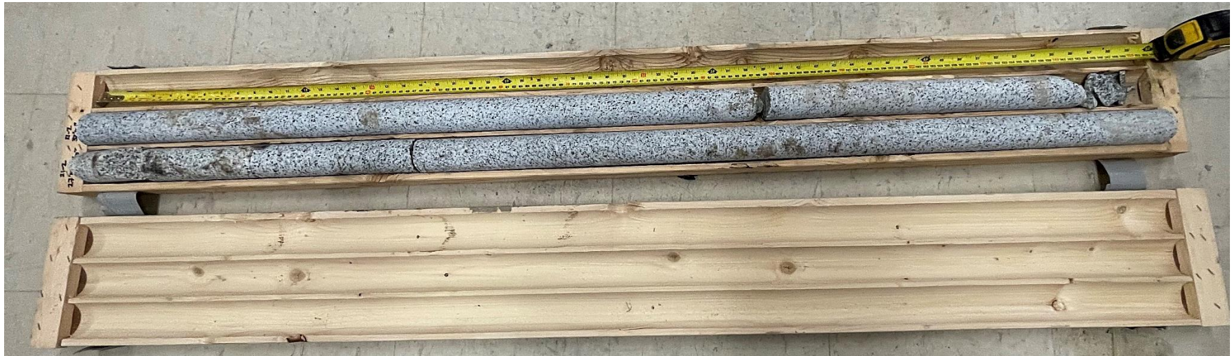
Figure E2. Rock core from BH21-2
