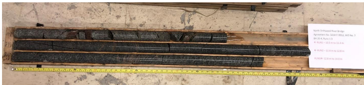
Photograph D2. Rock cores from BH20-4
