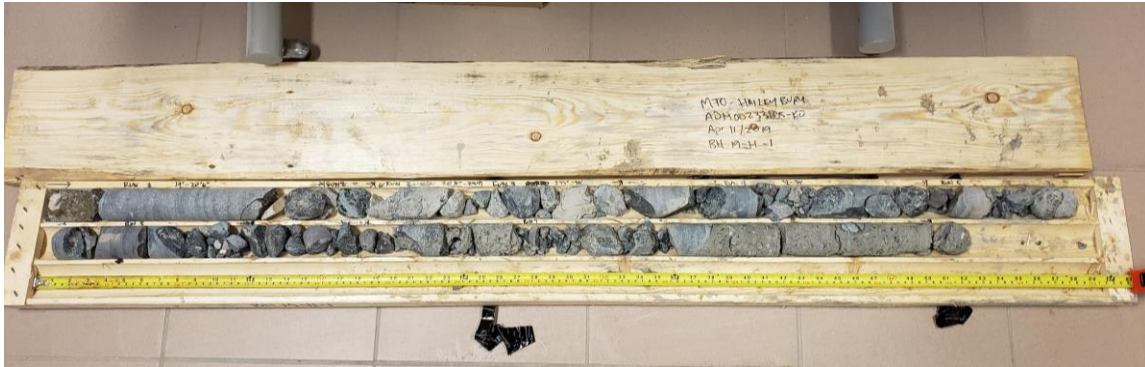
Photo 5: Sand and Gravel Till Cores with Cobbles and Boulder from BH19-H-1
