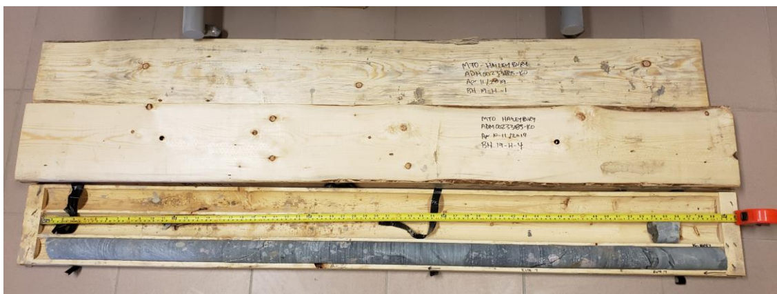
Figure E1. Rock core from BH19-H-4B
