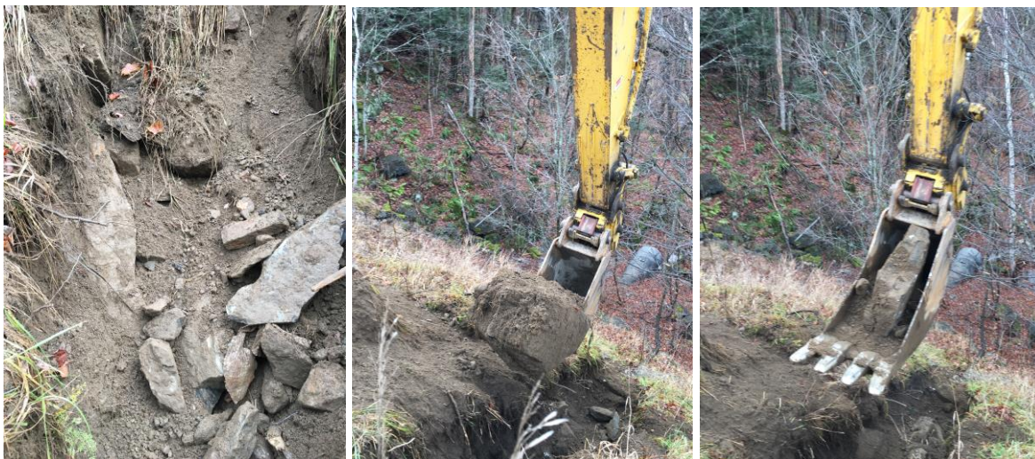
Photo 16: Test pit TP1 at the west embankment slope, various sized rock fragments in soil matrix
