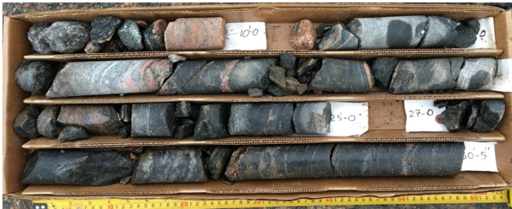
Photo 1. Rockfill Core Sample for BH201 from Elevation 348.4 m to 341.83 m
