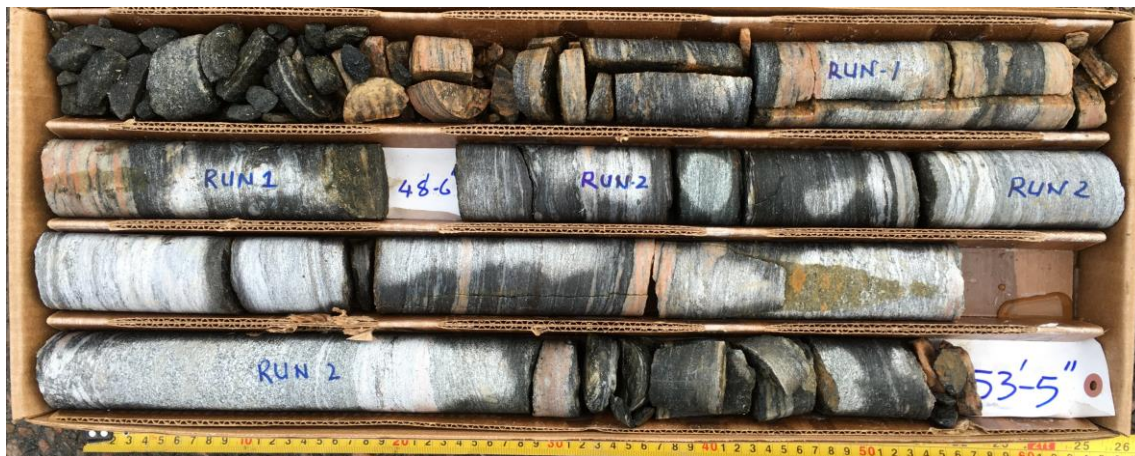
Photo 3. Bedrock Core Sample for BH201 from Elevation 337.6 m to 334.8 m
