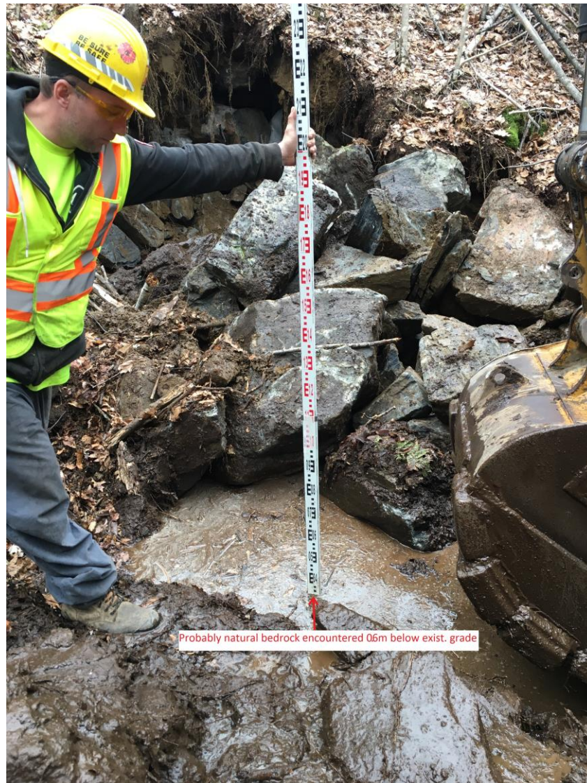
Photo 26: Test pit TP4 at the toe of the east embankment side, bedrock elevation
