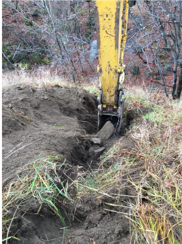
Photo 15: Test pit TP1 at the west embankment slope facing outlet side
