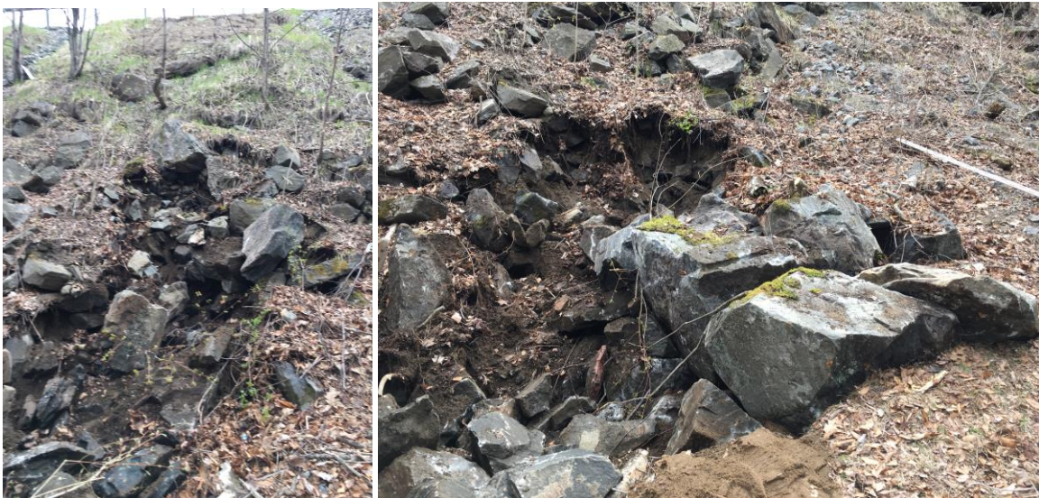
Photo 21: Test pit TP3 at the toe of the west embankment side, cobble and boulder sized rock fill
