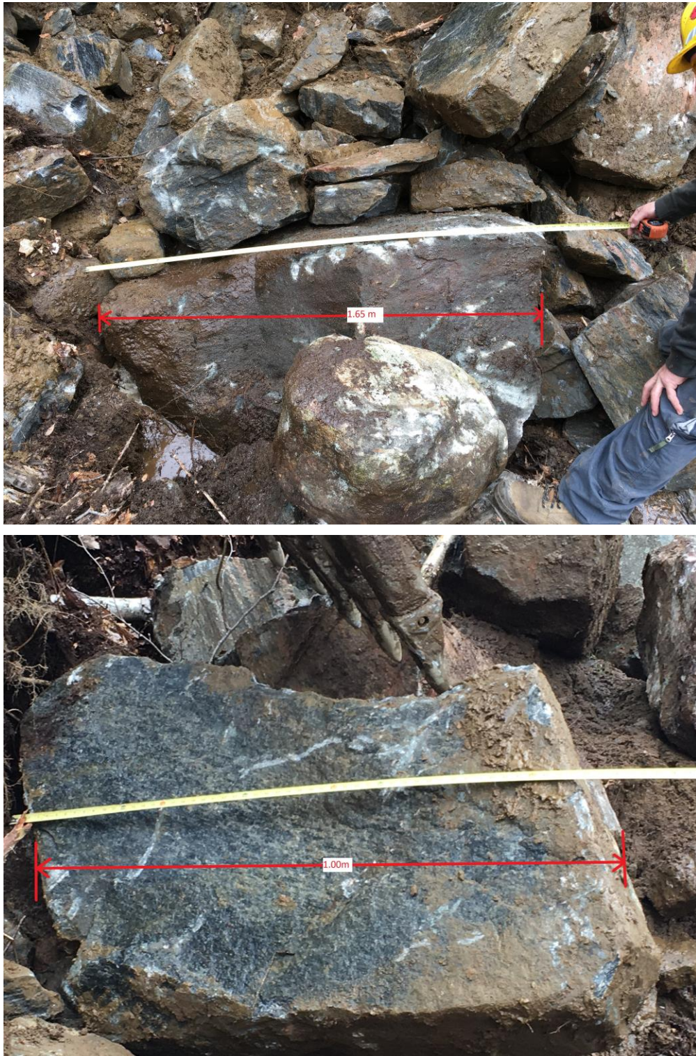
Photo 25: Test pit TP4 at the toe of the east embankment side, boulder sized rock fill
