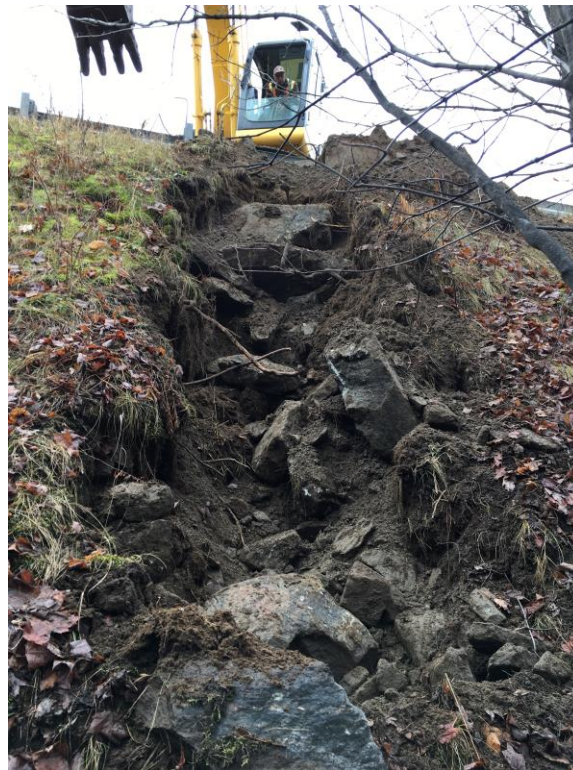
Photo 18: Test pit TP2 at the east embankment slope, various sized rock fragments in soil matrix
