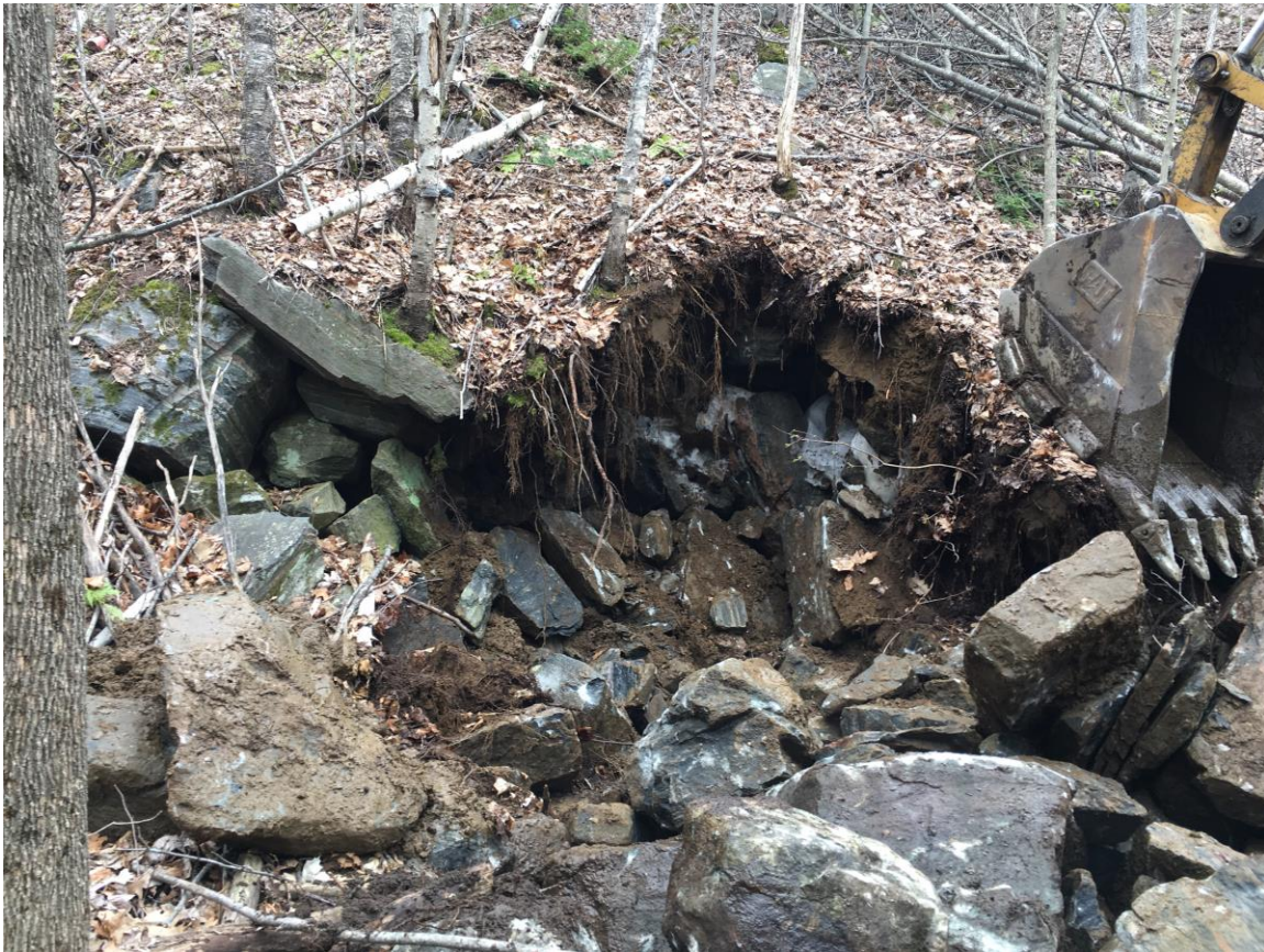
Photo 24: Test pit TP4 at the toe of the east embankment side, cobbles and boulder sized rock fill
