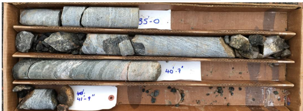
Photo 2. Rockfill Core Sample for BH201 from Elevation 341.83 m to 338.4 m
